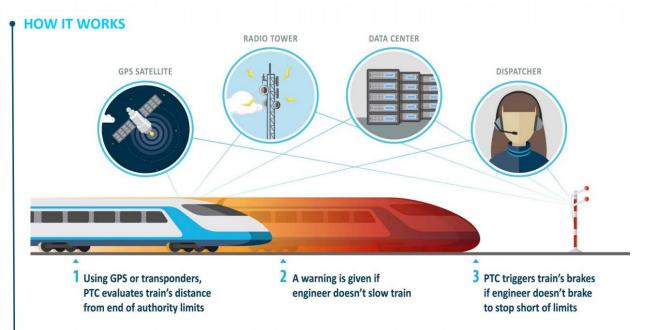
For example, PTC can force a train to stop before it passes a signal displaying a stop indication, or before running through an improperly lined switch, averting a potential collision.
