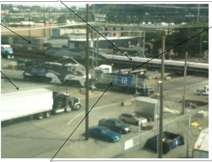
Amtrak switch engine pulling Sound Transit loco for maintenance
