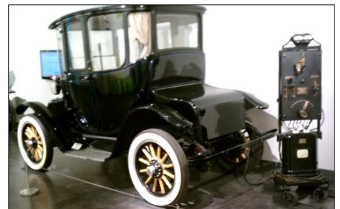
The 1914 Detroit Electric produced by the Anderson Electric Car Company. The device to the right is the charging station. Price when new $2,500-$3,000 (on display at the LeMay-America's Car Museum, Tacoma)
